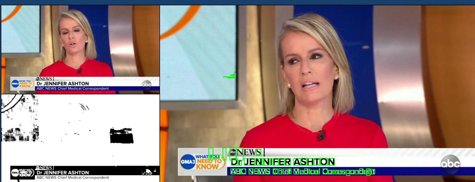
Original image (top left), result of pre-processing/morphology (bottom left), and detected text after passing through Tesseract OCR (right)
